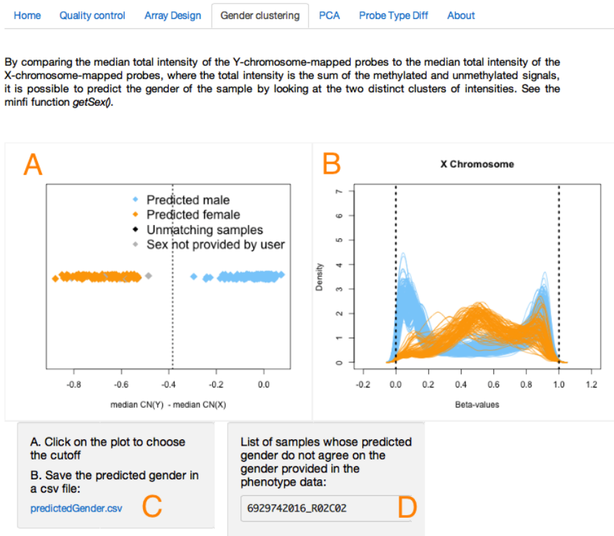
Figure 3: Sex prediction algorithm panel The difference of the median copy number intensity for the Y chromosome and the median copy number intensity for the X chromosome can be used to separate males and females
